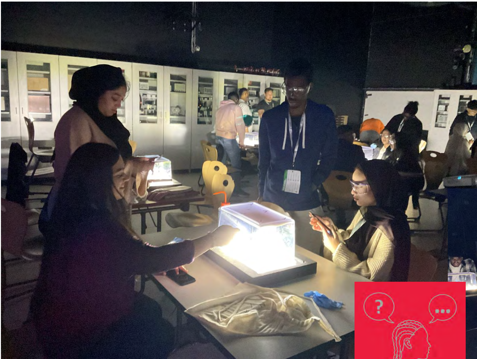
CERN SCool Laboratory – Cloud chamber experiment, investigating the formation of particles and how photons behave
